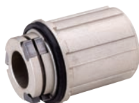
Shimano Freehub Body 8/9/10/11s Cassette 3 PAWLS AL 7075 Sealed Bearings \varnothing 12/\varnothing 15 \varnothing 12 B52R/B56R \varnothing 15 B63R/B64R/B65R/B66R
